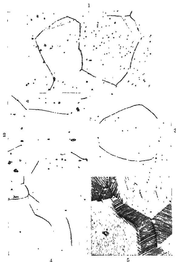
(1) COPPER-BERYLLIUM ALLOY, ELECTROLYTICALLY POLISHED, CHEMICALLY ETCHED. \times 1,000 (2) ALUMINIUM-MAGNESIUM ALLOY, ELECTROLYTICALLY POLISHED, CHEMICALLY ETCHED. \times 500 (3) COPPER-BERYLLIUM ALLOY, ELECTROLYTICALLY POLISHED, CHEMICALLY ETCHED. \times 750 (4) SILVER, ELECTROLYTICALLY POLISHED, THERMALLY ETCHED IN NITROGEN. \times 200 (5) SILVER (SAME FIELD AS 4 AFTER SUBSEQUENT HEATING IN AIR). \times 200
